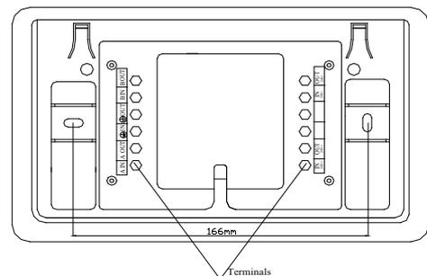
The system cables connect to the base, and linked to the repeater by internal cables.
